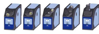
The operating distance is measured starting from the lens front face. The reading direction can be changed inverting the cap and lens. Mark detection on a reflective surface is improved adjusting the beam direction to 5° ... 20° from surface axis.
